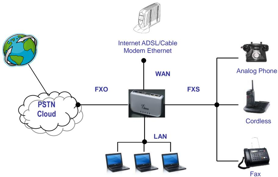
**FIGURE 2: INTERCONNECTION DIAGRAM OF THE HT503**
